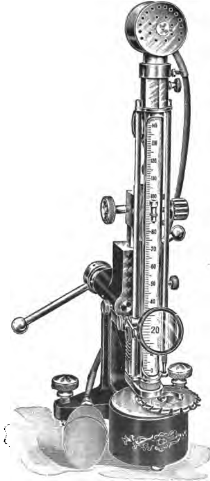
Fig. 187. Scleroscope Testing Set Courtesy of Shore Instrument Company, New York City
